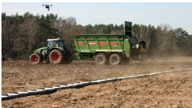
Fig. 2: The mobile test stand for measuring the distribution across rows
