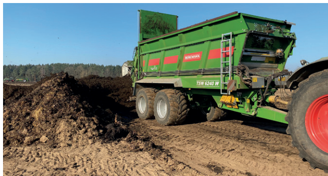
Fig. 3: BERGMANN TSW6240 W with V-Spread is unloading the material during the measurements on application along rows
