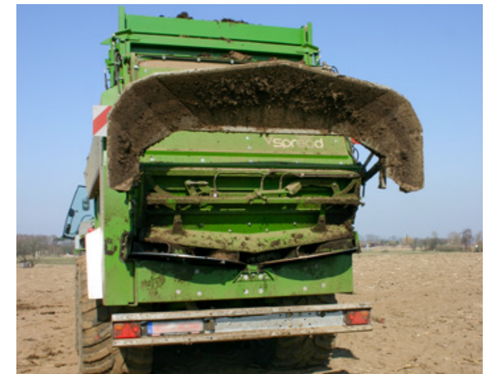
The V-Spread spreader unit with spreader disks of 1,100 mm diameter and six spreader blades.
