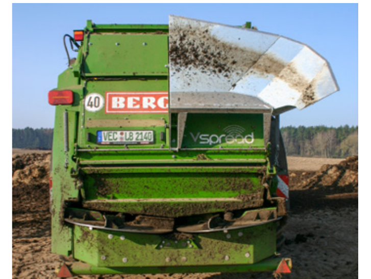
The V-Spread spreader unit with spreader disks of 1,000 mm diameter and four spreader blades.
