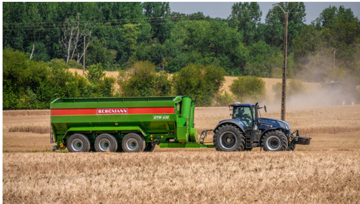
GTW 430 With a load volume of 43 m 3 , the GTW 430 is the flagship of the BERGMANN Transfer Trailers. The transfer rate is about 1,100 t/h.
