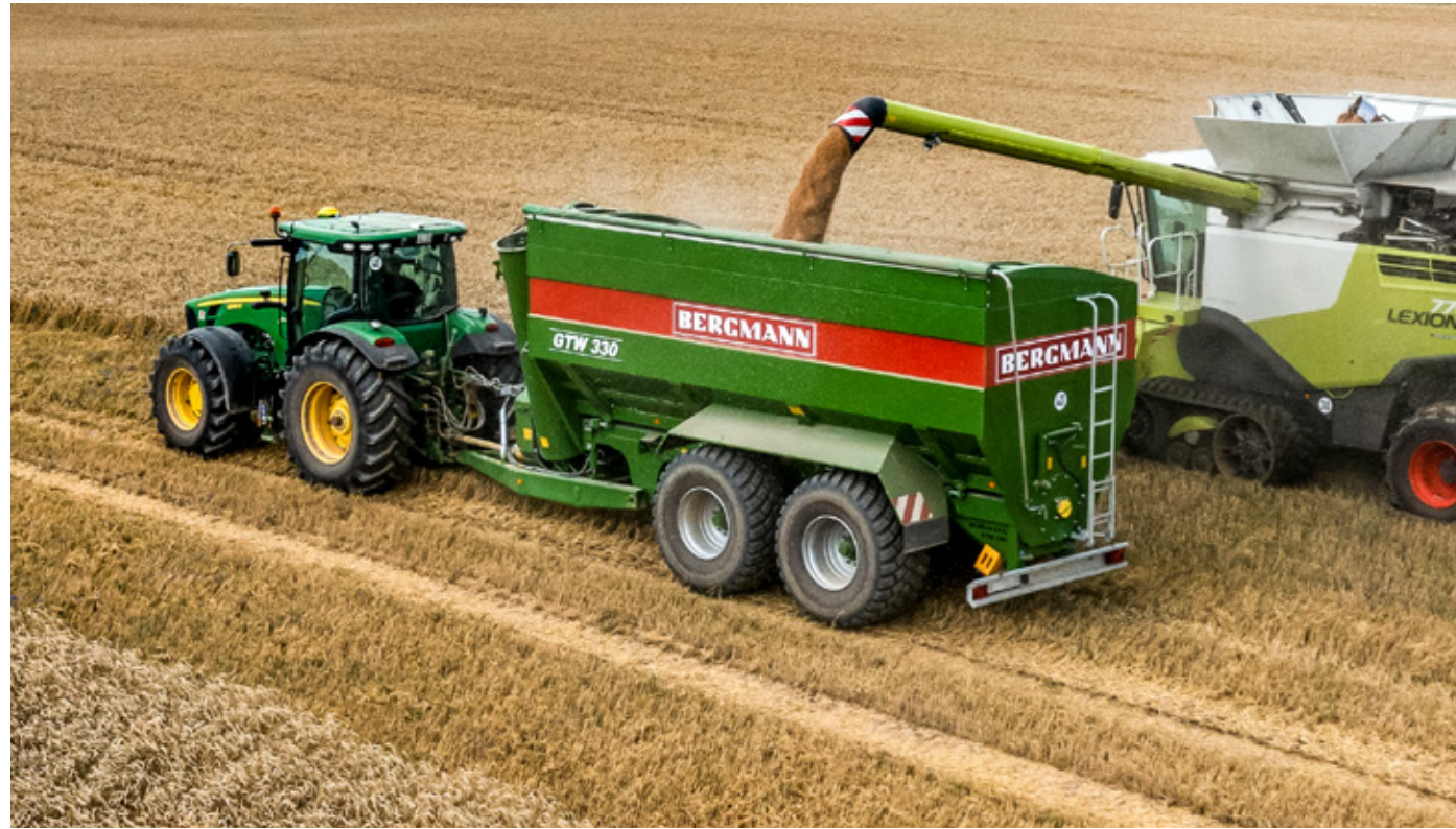
GTW 330 With a load volume of 33 m 3 , the GTW 330 belongs to the top range of BERGMANN Transfer Trailers. The transfer rate is about 1,100 t/h.
