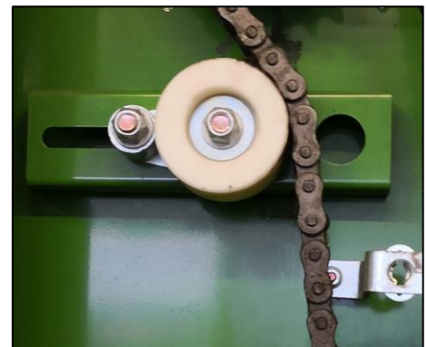
Image 165: Chain tensioning block
