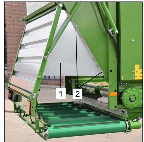
Image 47: Removing the cover plates
