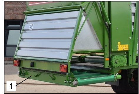
Image 39: Cross conveyor belt
