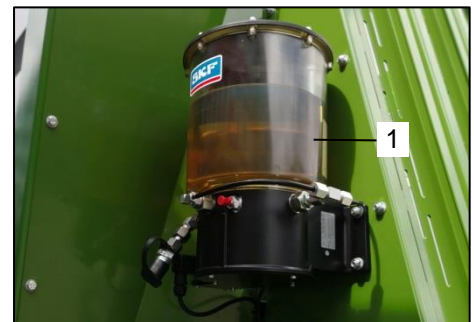
Photo 53 : Installation de lubrification
