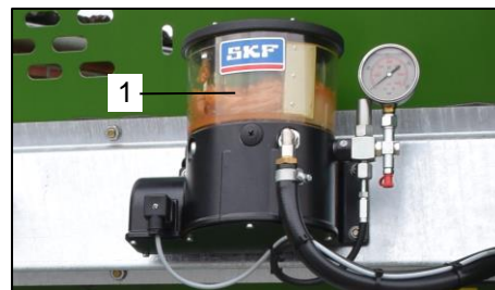
Photo 57 : Installation de lubrification
