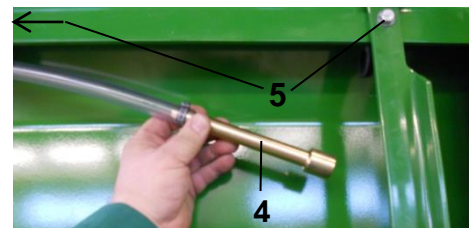
Photo : Retirer le tube de raccordement
