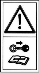
Mount and dismount the PTO shaft only when the motor is off and the ignition key has been removed!
