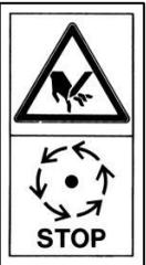
After the power has been switched off the unit can continue to run due to momentum. During this time, keep a safe distance. Only when the drive has come to a complete stop, may it be approached!
