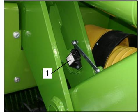
Fig. 10: Drawbar Sensor, Right
