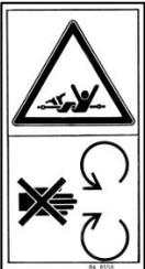
When working on the PTO shaft itself, no one should be in the area of the rotating PTO shaft!
