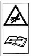
Hydraulic oil, which leaks out under high pressure, can penetrate the skin and cause serious injury! In case of injury, notify a doctor immediately. Danger of infection!
