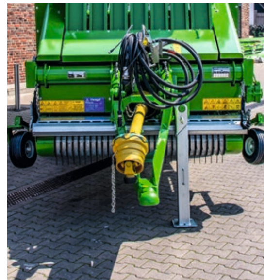
The narrow drawbar design ensures high manoeuvrability and low wear. The jack stand can be swivelled up and fastened to the frame.
