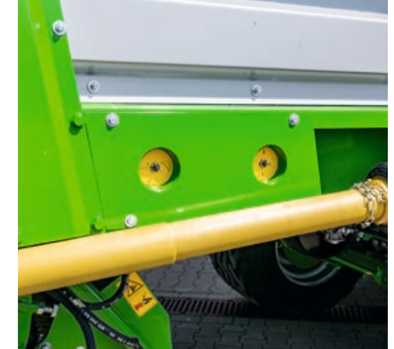
The drawbar and knife beam can be easily adjusted on the left side of the vehicle.
