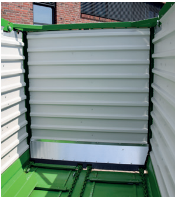
K-model without dosing rollers ( CAREX 390 K / CAREX 430 K )
