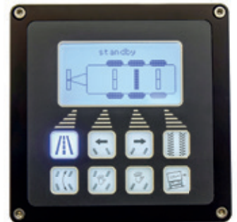
Control panel for the electro-hydraulic forced steering
