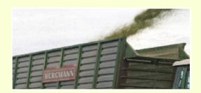
The upper section of the front (600 mm) wall can be folded down for interference free filling.
