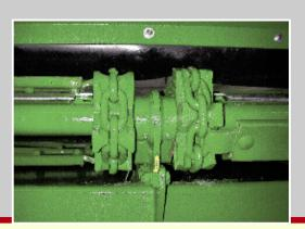
Four high-strength  $14 \times 50$  mm round steel chains with an overall tensile strength of  $4 \times 25$  t = 100 t, on which solid scraper floor bars are bolted, provide for high durability and functionality, even under continuous load.
