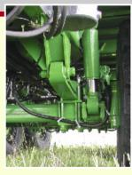
Hydrostatic suspension. The load is distributed evenly on all wheels. The suspension travel distance of up to 300 mm guarantees top handling on uneven ground.
