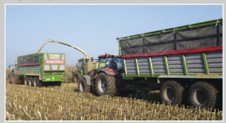
All Forage Transport Trailers are optionally available with a hydraulically operated cargo space cover.
