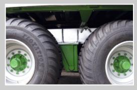
The pivoting point of the parabolic springs of the Boogie chassis lies beneath the axle or the center point of the wheel. This optimises driving comfort even under difficult road conditions and heavy loads. The easy to pull chassis makes it easier to pull the vehicle over obstacles.
