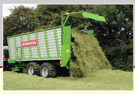
The bin has a tapered design to provide for quick unloading of the forage transport trailer. The trailer is emptied down to the last bit in approx. one minute.
