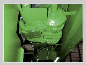
The scraper floor is driven mechanically from both sides (with two dosing rollers). If the HTW is without dosing rollers, the scraper floor is driven hydraulically from both sides (mechanically upon request).
